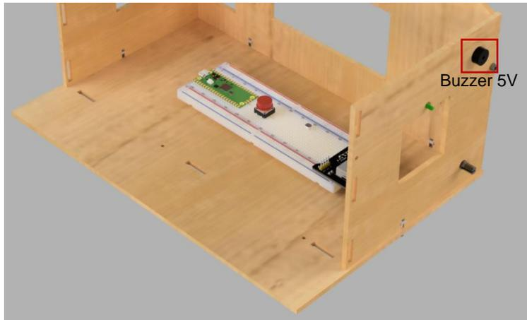
2. Place the push button on the breadboard.
