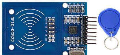
Figure 4 RFID Reader RC522
