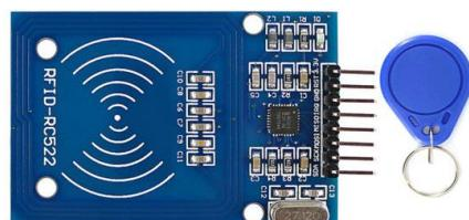
Figure 4 RFID Reader RC522
